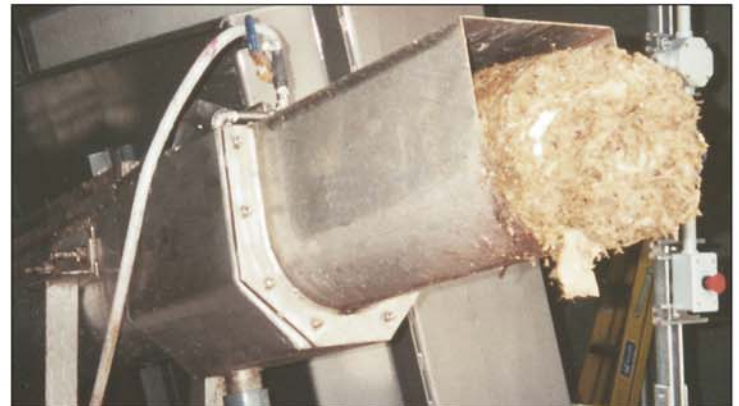
WTP EQUIPMENT CORP. MECHANICAL BAR SCREEN DISCHARGING TO A SCREENINGS WASHING DEWATERING PRESS
